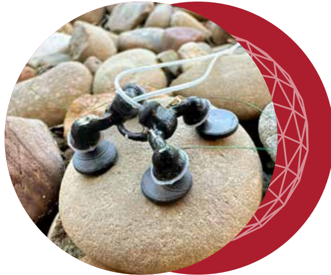
This combustion-powered quadrupedal robot is capable of multi-gait movements and can leap 60 centimeters in the air, or roughly 20 times its body length.
