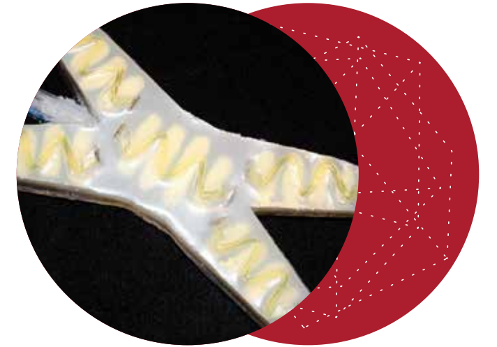
Researchers installed SHeaLDS – self-healing light guides for dynamic sensing – in a soft robot resembling a four-legged starfish and equipped with feedback control. After the researchers punctured one of its legs, the robot was able to detect the damage and self-heal the cuts.
