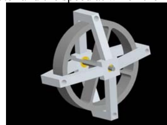
Fig. 2. The basic CMG design including the rotor and gimbal casing.
