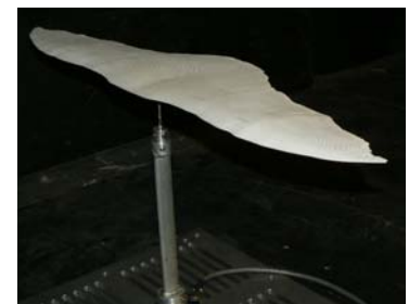
Rigid bat wing test setup in wind tunnel
